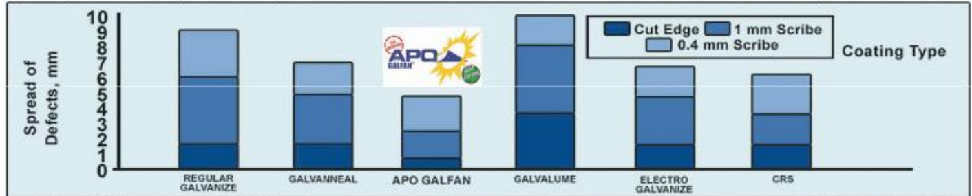
Figure 2 - Spread of defects after 2 years in industrial exposure.
